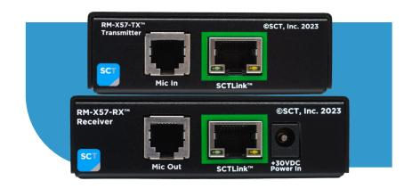
Sound Control Technologies (SCT) Microphone Extension Kits are designed to bring you the microphone inputs from the Poly Studio, X50, or X70 backplane right to the *table*!
