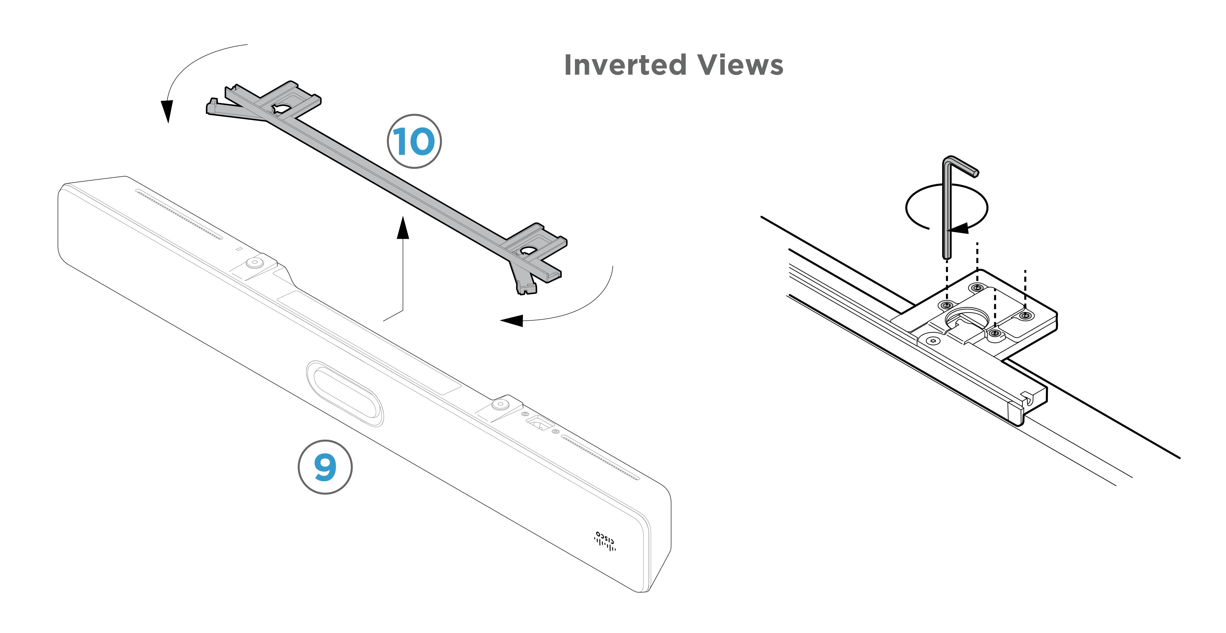
STEP 5: Place camera on bracket assembly and pivot locking tabs back flush into place.
